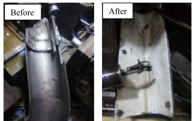
Figure 3- Comparison of Metallic Output Chute and PP Layer Modification
