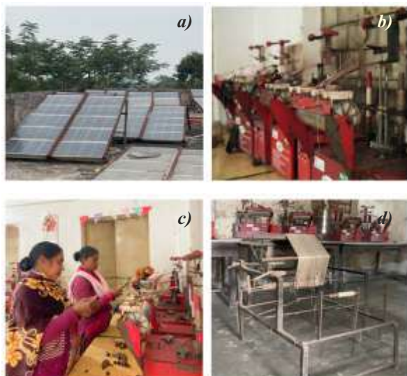
Figure 14: a) Solar panels, b) Reeling-cum-twisting-machine, c) Reeled yarn making, d) Re-reeling machine
