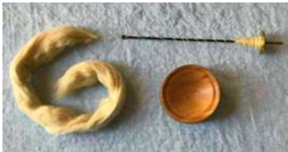
Figure 1: Takli used for spinning cotton Khadi
