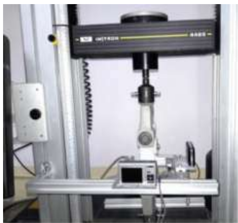
Figure 1: set up on INSTRON for determination of Poisson's ratio of nonwoven samples
