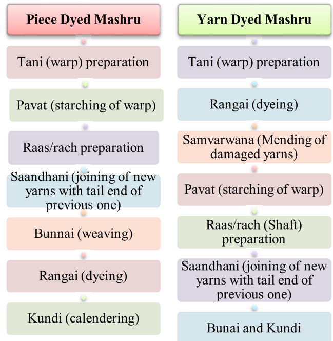
Figure 6 - Manufacturing process of Piece Dyed Mashru and Yarn Dyed Mashru
