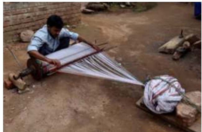
Figure 4: Beaming process for warping
