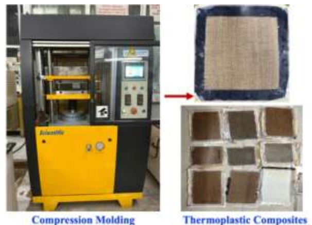
Figure 2. Manufacturing Process of 2D woven fabric-based thermoplastic composites
