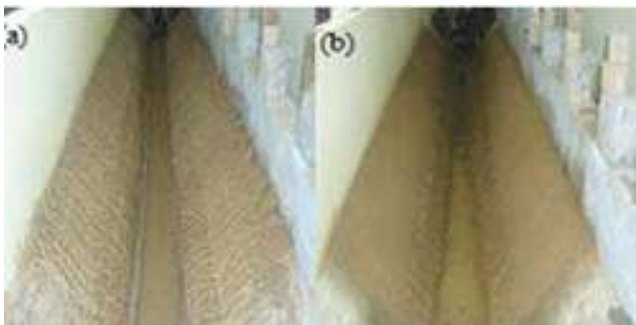
Figure 5 : River model with geotextile mat and cocolog (a) before experiment (b) after experiment
