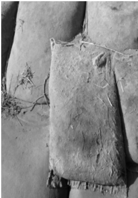
Figure 1: Different types of Geobags placed as temporary wave protection.
