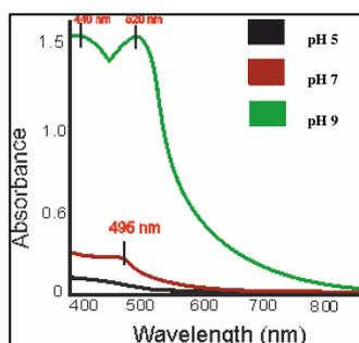
**Figure 1- Visible spectra of dye extracted from *Peepal* bark in aqueous medium at varying pH**
