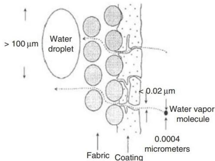
**Figure 5 - Schematic representation of moisture transfer through porous coating**
