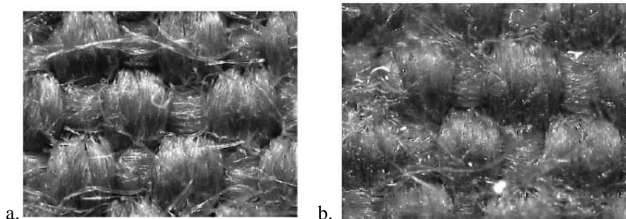
**Figure 1 – a) dry (Ventile fabric), b) wet** (Curtesy: Woodhead Publishing Ltd.) [2]
