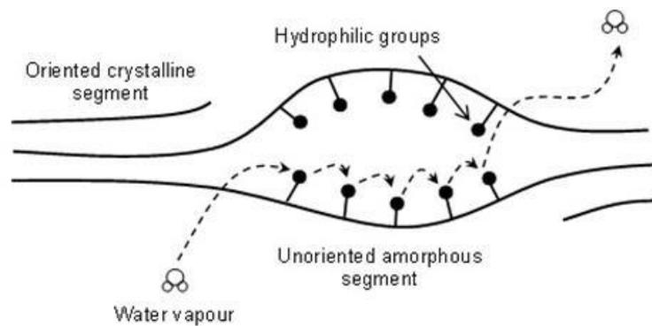
**Figure 3 - Schematic representation of moisture diffusion through hydrophilic membrane [1]**
