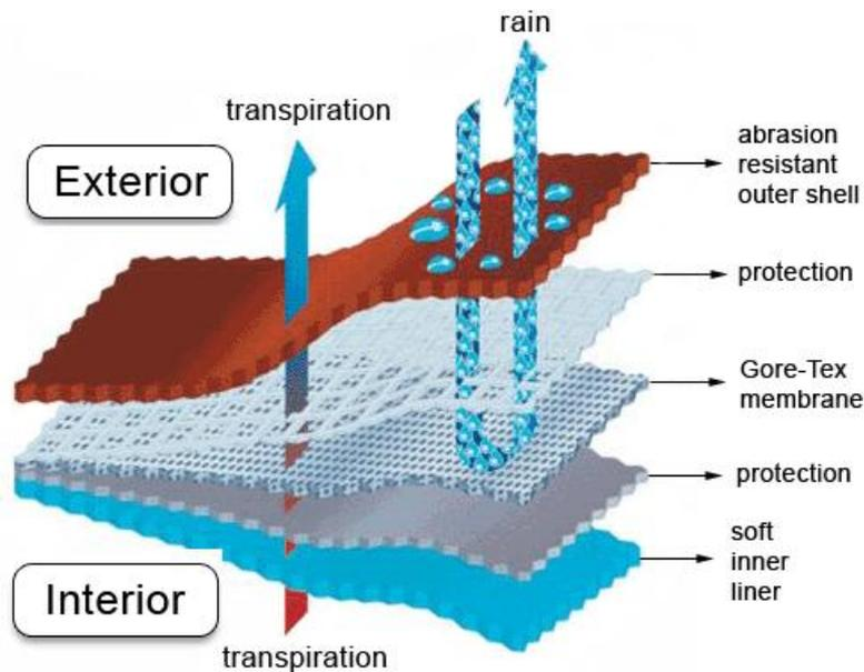
**Figure 2 - Moisture transfer through membrane: Gore-Tex® construction**
