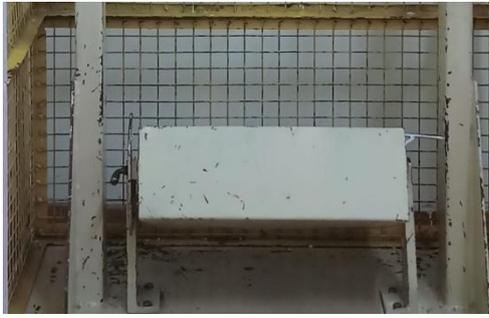
**Figure 4 - Box provided with gear system to adjust the angle of incidence**
