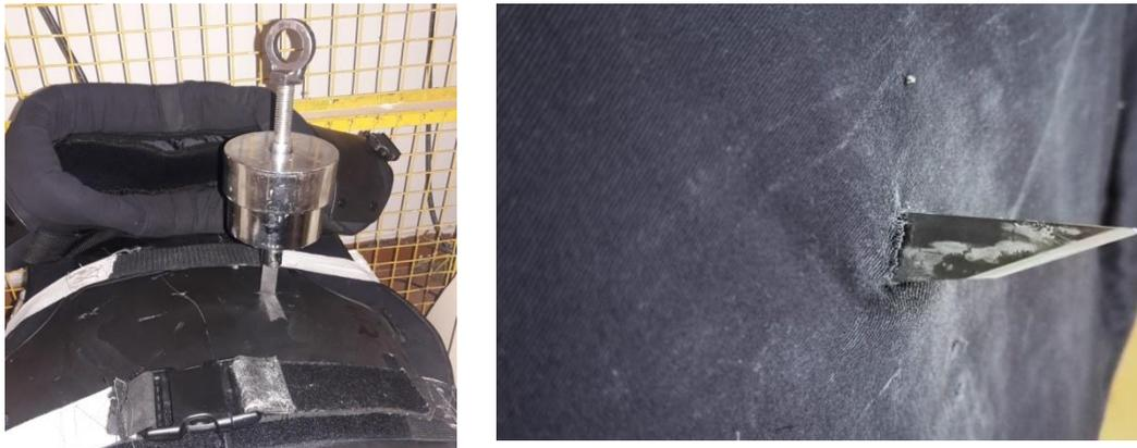
**Figure 10 - Performing stab test on body protector**
