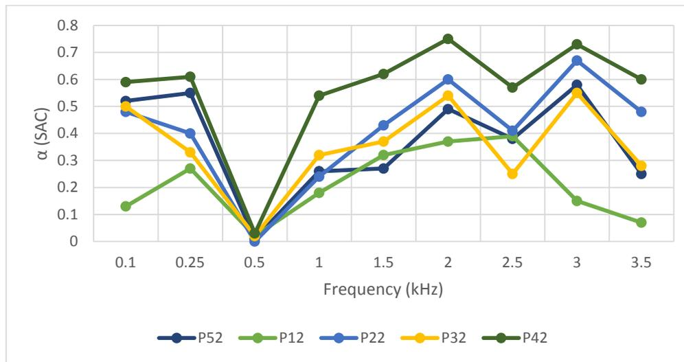
**Figure 4:** Acoustic behavior of double layer nonwoven composites
