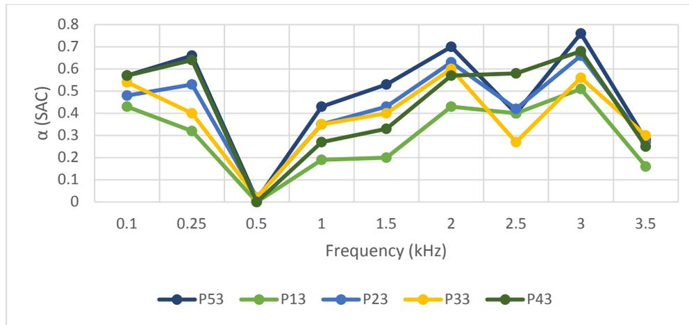
**Figure 5: Acoustic behavior of triple layer nonwoven composites**
