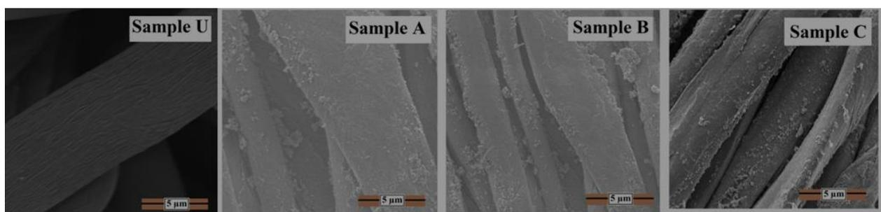
Figure 3 - SEM images of copper oxide coated cotton fabric
