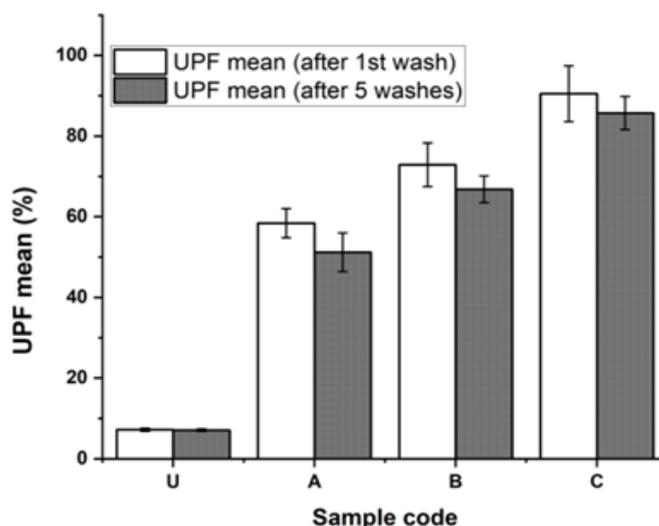
Figure 1- UPF mean of copper oxide coated fabric
