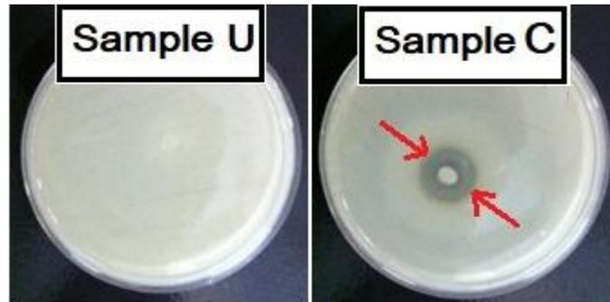
Figure 2- Images of zone of inhibition of untreated and copper oxide treated fabric (Against Gram positive bacteria)
