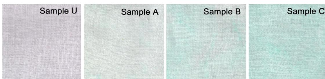
Figure 4- Photographic images of untreated and copper oxide treated fabric samples
