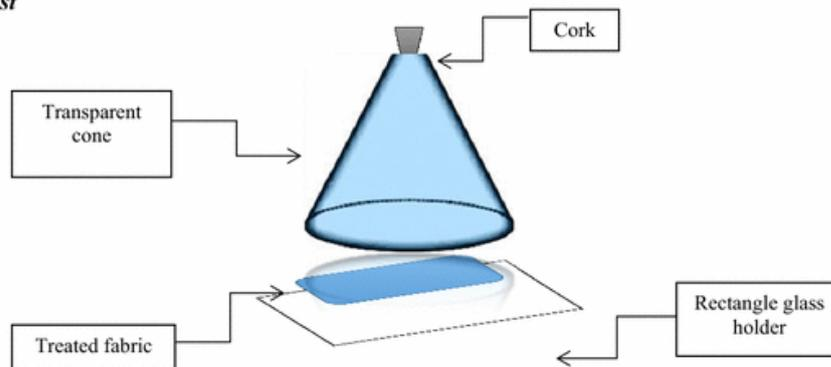
Figure 3: Cone Test
