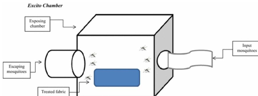
Figure 4: Excito Chamber Test
