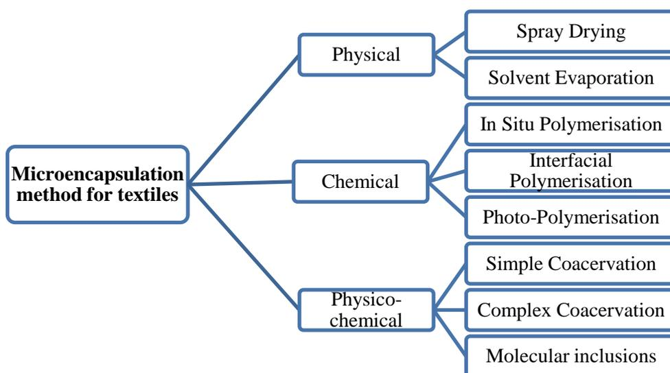
**Figure1- Microencapsulation methods used in Textiles**
