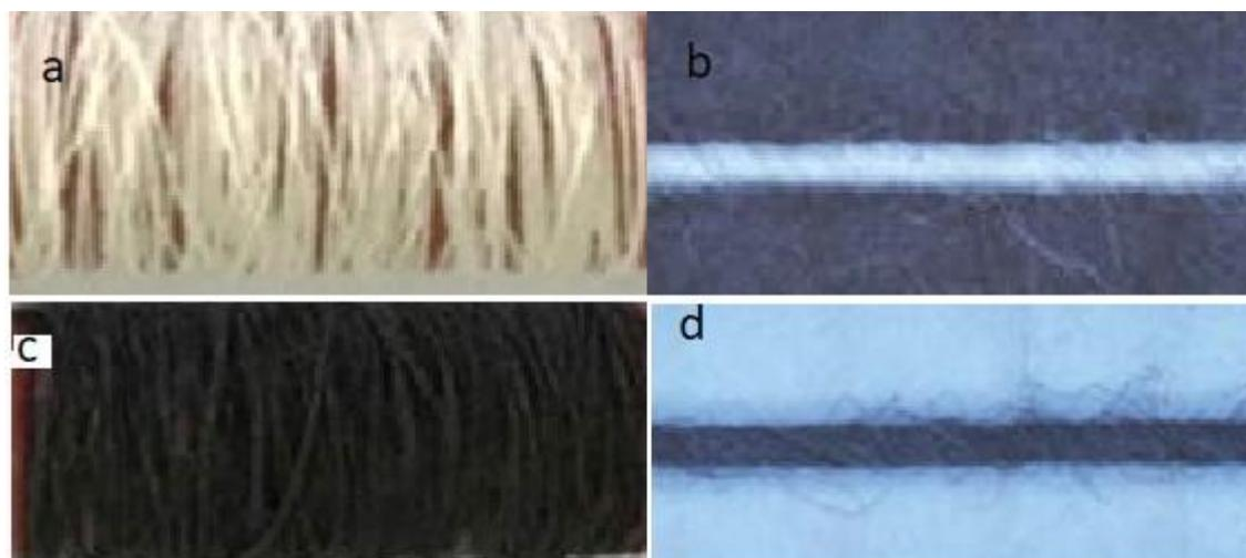
**Figure 1 - (a. Woolen bobbin, b. Woolen thread, c. poly-pyrrole coated bobbin, d. poly-pyrrole coated thread)**
