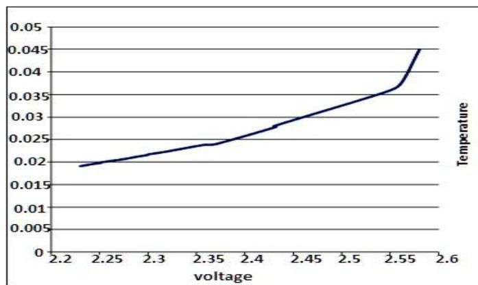
**Figure 3 - Voltage Temperature characteristics of conductive thread**
