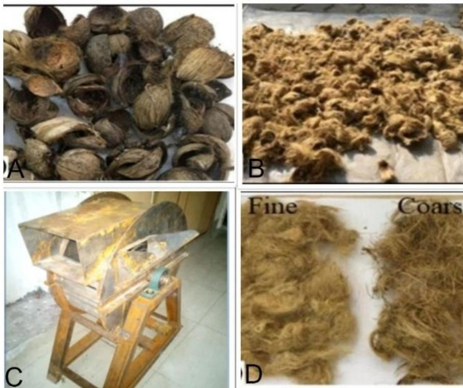
Figure 5 - A: - Areca sheath B: - Softened Areca sheath C: - Areca Extraction machine D: - Extracted Areca fibres
