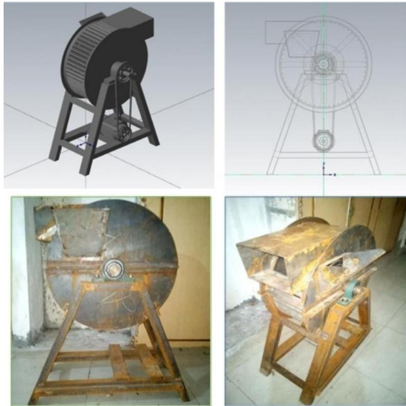
Figure 4 - Different views of the Areca Extraction machine
