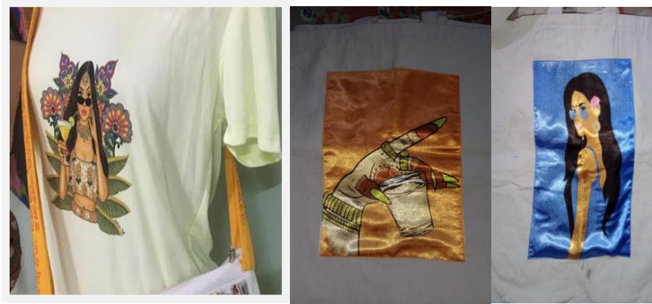
Figure 2 – Physical prototypes developed using Sublimation printing
