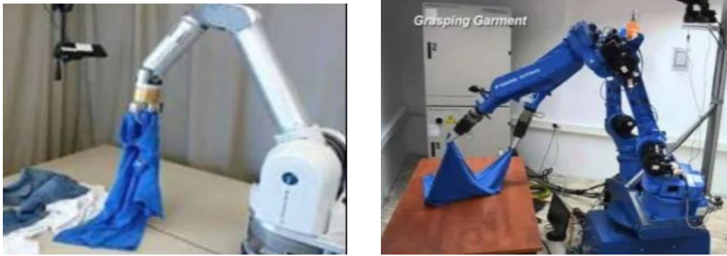
Figure 5 - Garment folding and Packaging by dedicated Robotic arms
